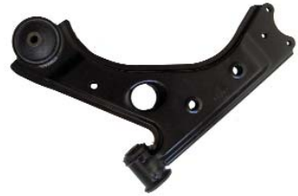
▶ Orj Ref : OP133-L Descr. : Lower control arm without ball joint-L OEM No : Note :
