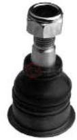
▶ Orj Ref : NS038 Descr. : Ball joint OEM No : 4016050J25-4016086M00 Note : M14*1.5 RHT
