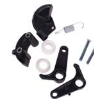
▶ Orj Ref : RN024 Descr. : Clutch pedal repair kit OEM No : 7700498487 Note : Kit
