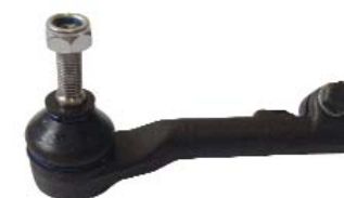
▶ Orj Ref : RN204-L Descr. : Tie rod end-L OEM No : 7701041311-7700834570-6000022752-7701470765 Note : M14*1.5 RHT
