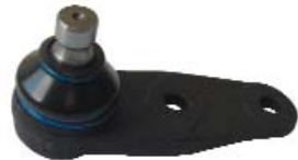
▶ Orj Ref : RN100 Descr. : Ball joint OEM No : 7701462182-7701468883-7701472038-7701468411-5450100QAH Note : Lower
