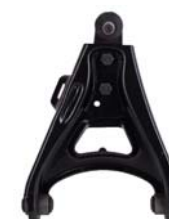
▶ Orj Ref : RN042-L Descr. : Lower control arm complete-L OEM No : 7700783453-7700783455 Note :
